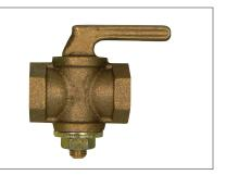
Brass body and plug manually operated low pressure natural or propane gas valve for use indoors on house piping system between the meter oulet and the inlet connection of the gas appliance at ambient temperatures of 32 to 125 degrees Fahrenheit.
